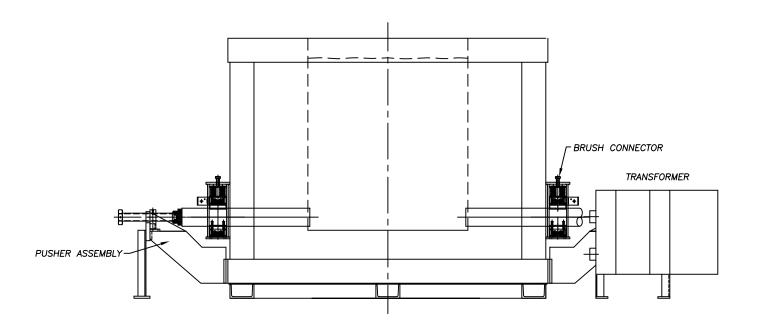
UPTON SUBMERGED GRAPHITE ELECTRODE SALT BATH FURNACE U-E
